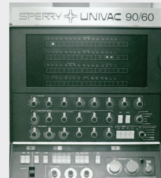
Like all mainframes in the 1960s to 1980s, the Sperry Univac 90/60 processor was large but held limited memory.
